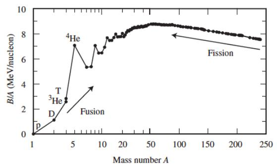
Figure 1: Binding energy per nucleon
