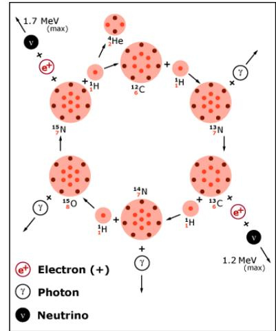
Figure 5: Schematic diagram of the CNO cycle.
