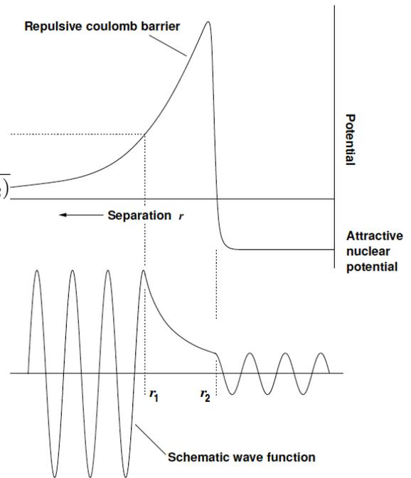
Figure 2: Top image shows schematic diagram of Coulomb barrier and the attractive strong force. Bottom image shows exponentially decreasing amplitude of wavefunction as nuclei tunnel through Coulomb barrier.
