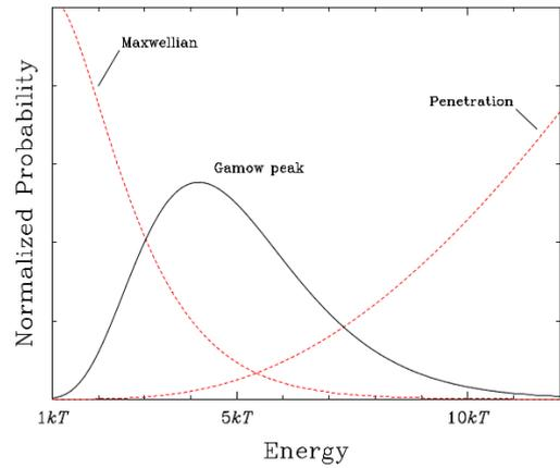
Figure 3: This figure illustrates the competing influences of the decreasing probability of having high energy particles in the Maxwell distribution, and the increasing probability of tunnelling at high energies, giving rise to the Gamow peak.
